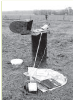
Sampling and water-level measurements in a standpipe
