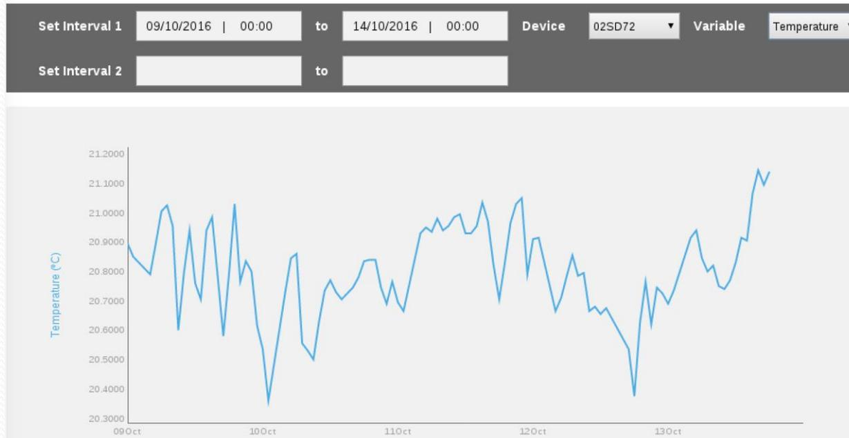
Current option allows user to define period of time, sensor and the sensor's variable to visualize. All sensors (of the selected dam) and correspondent variables currently registered on the Energy DSS are able to be visualized.
